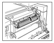
8 Fully move the two lock release levers for the oil-coating unit in the direction of the arrows.
